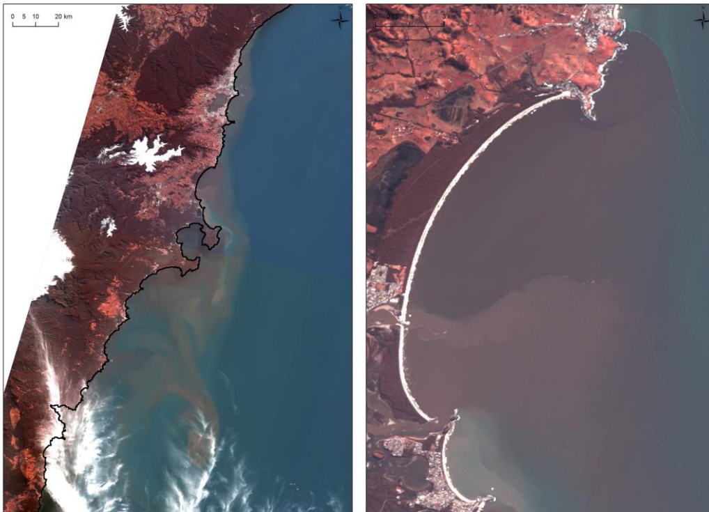
Fig. 6: 30/06/2013 Landsat 8 false colour composite showing breached Shoalhaven Heads transporting fine material out of the primary compartment, towards both north and south directions.
